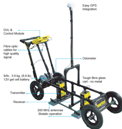
Figure 7. A picture with labels of the GPR instrument and smart kart used to acquire GPR data.
