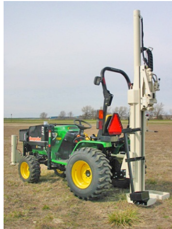
Figure 9. A picture of the Geoprobe Model 54TR rig mounted on the rear of a John Deere 420 tractor used to extract cores similar to the one used in the study.
